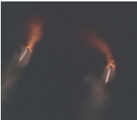
Figure 2. Space Shuttle SRB slag emission at SRB separation +30.5 sec. Chamber pressure < 6.9 kPa. Numerous Tail-off ejecta are clearly resolved as the plume brightness fades. Ejecta continue to stream from the SRBs, although at a reduced rate, for several minutes.
