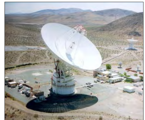
Figure 1. The Goldstone radar transmitter dish (foreground) and receiver dish (background). In this photo, the antennas are not pointed for orbital debris data taking.
