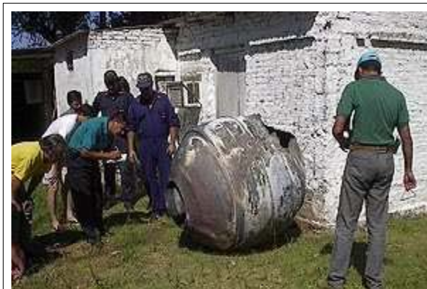
Titanium casing of the STAR-48B solid rocket motor found in northeastern Argentina.
