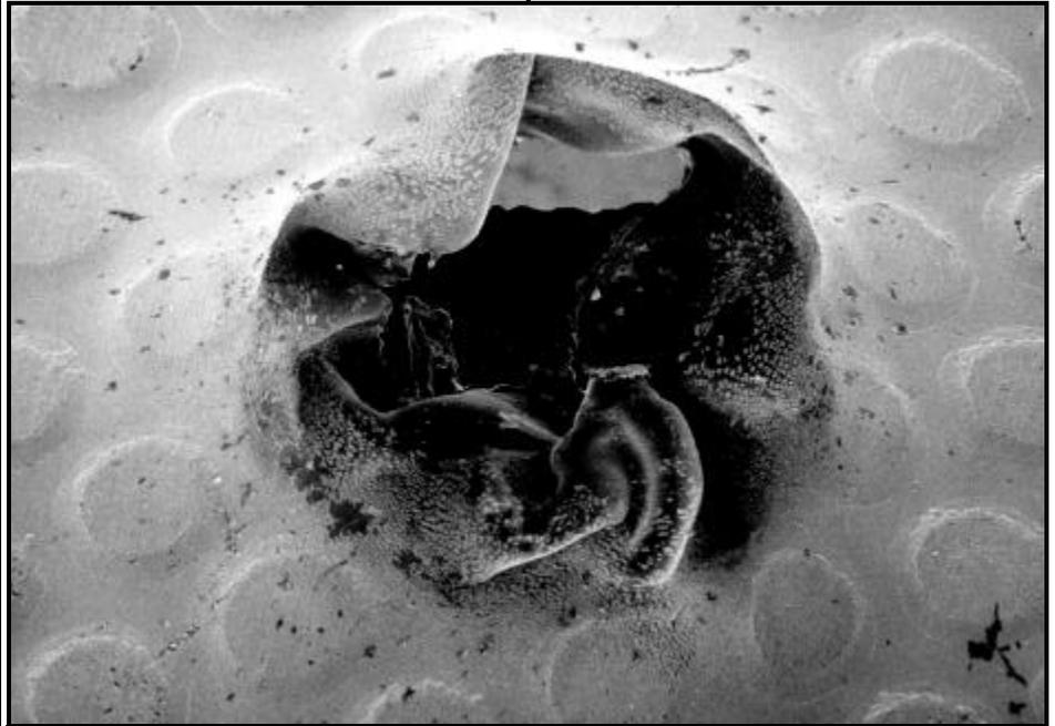
Figure 1. SEM image of a radiator impact and through face sheet penetration (sample 50).
