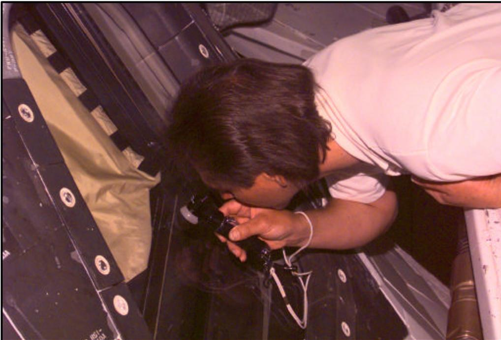
**Figure 2.** A magnifier with light source is used to examine small impact regions on a thermal pane of the Space Shuttle.
