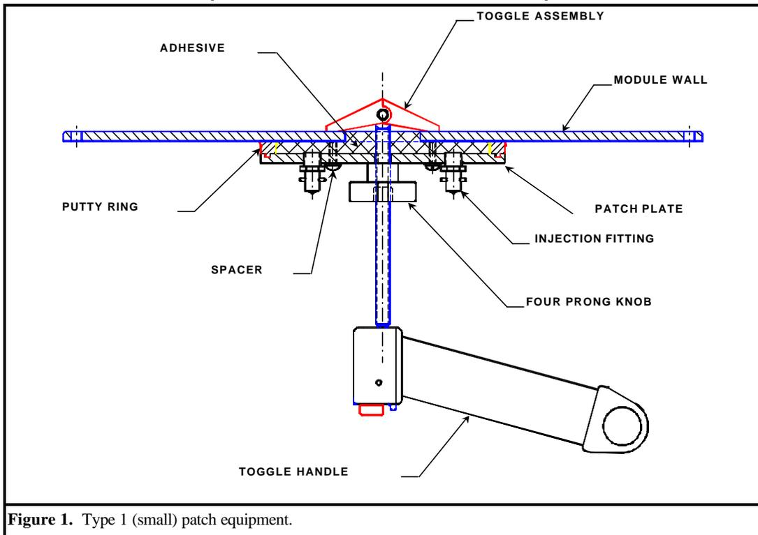
Figure 1. Type 1 (small) patch equipment.
