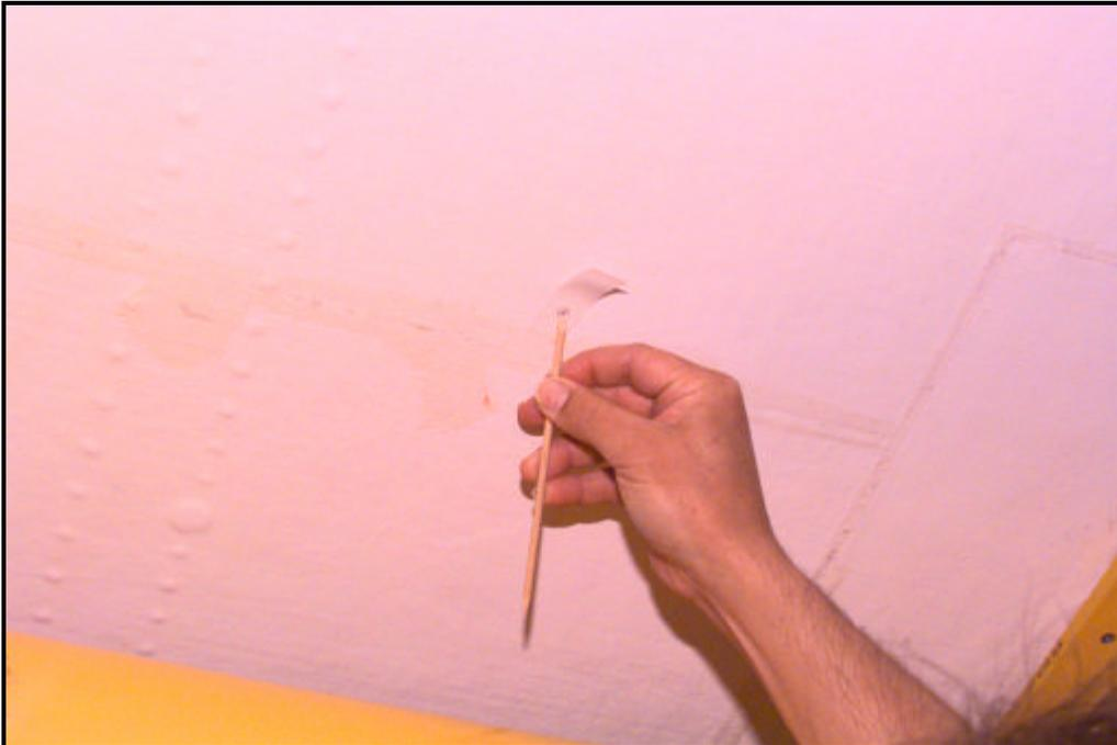
**Figure 1.** A probe and adhesive tape are used to retrieve residue inside a crater in the FRSI caused by an orbital debris or meteoroid impact.
