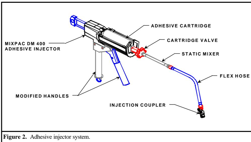
Figure 2. Adhesive injector system.
