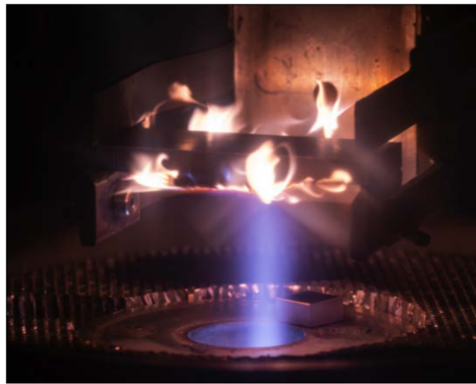
Figure 1. Image of carbon fiber-reinforced polymer sample coupon under test at the University of Texas Inductively Coupled Plasma (ICP) Torch Facility. Courtesy of Colin Yee, graduate student on the UT project, reproduced with permission.
