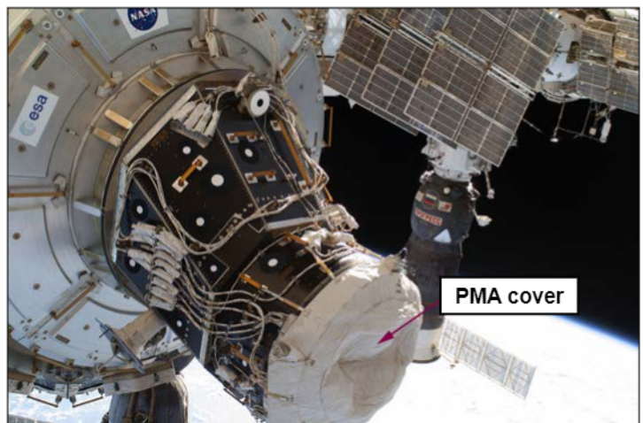
Figure 1. The ISS Node 3 axial port’s PMA-3 cover. The PMA-2 cover, on the Harmony module’s PMA, is otherwise identical, though no on-orbit imagery appears to exist. Credit: NASA photo #iss035e037061
