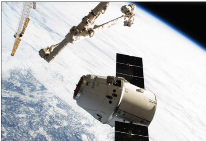
Figure 3. The SpaceX Dragon capsule flown on the Commercial Resupply Mission 17 (CRS-17). The conical capsule's lateral surface is SPAM TPS material. Credit: NASA photo #iss059e043284
