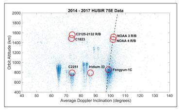
Fig. 2. Conversion of HUSIR range and range-rate measurements into altitude and Dopplerderived inclination. The sun-synchronous condition, assuming a circular orbit, is indicated with the dashed black line.
