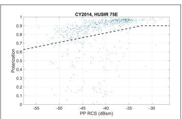
Fig. 6. Identification of the piecewise linear line that separates the NaK from the rest of the orbital debris population with altitudes < 1000 km and Doppler inclinations between 62.9° and 67°. The polarization shown is limited to positive values to highlight the NaK population, which has polarizations near unity.
