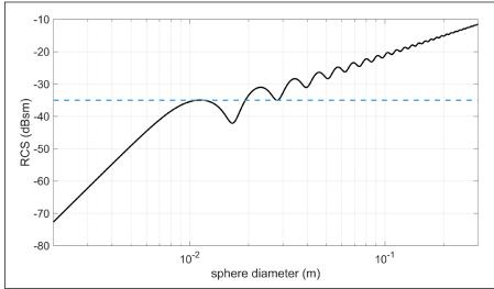
Fig. 8. Mie sphere scattering for the HUSIR X-band wavelength. A reference line at -35 dBsm marks the inflection of the RCS curve where a sudden increase in the NaK cumulative count rate is expected for HUSIR X-band operation.
