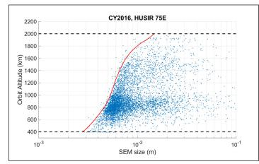
Fig. 5. Orbital debris observations in altitude and SEM-size space for the 2016 HUSIR 75E data. The red curve indicates the altitude and SEM-size sensitivity relationship for the radar in 2016. Dashed black lines indicate approximate altitude limits for the HUSIR orbital debris mode.
