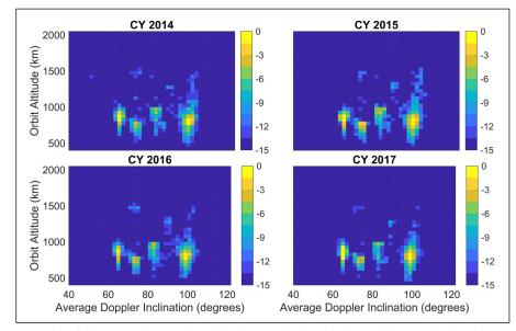
Fig. 3. Orbital debris count density in altitude (km) vs. Doppler-derived inclination (°) space. The color scale is in decibels (dB), hence each 3 dB decrease represents a factor of 2 decrease in count density.
