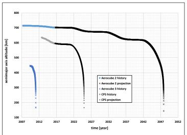
Figure 3. A comparison of the projected future evolution of the semimajor axis altitude for AeroCube 2 and CP5. The NASA Orbital Debris Program Office (ODPO) standard computer tools and models were used to estimate the historical area-to-mass ratio of these spacecraft and propagate them into the future. The latest Debris Assessment Software (DAS) solar activity file was used to model expected solar activity over the next five decades.
