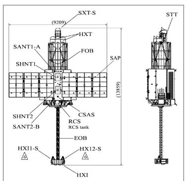
Figure 1. An exterior view of the ASTRO-H spacecraft (from Ref. 1). All dimensions are in millimeters. Relevant acronyms are Solar Array Paddles (SAP); Extensible Optical Bench (EOB), and Reaction Control System (RCS). See Ref. 1 § 2.3 for a complete list of acronyms.
