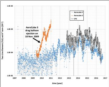
Figure 2.  $B^*$  time history for CP5 and AeroCubes 2 and 3. The AeroCube 3 history is consistent with that presented in Ref. 2. AeroCube 3 was launched to a much lower altitude than the other two spacecraft but this does not account for the secular growth of  $B^*$  over time.
