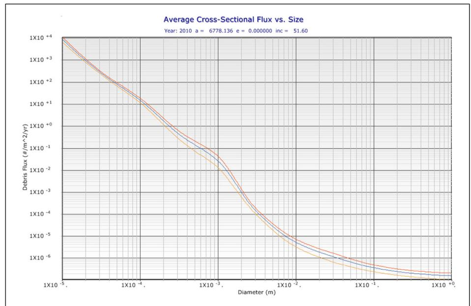
Figure 1. ORDEM 3.0 ISS debris diameter vs. cross sectional flux, with error bars (GUI output).
