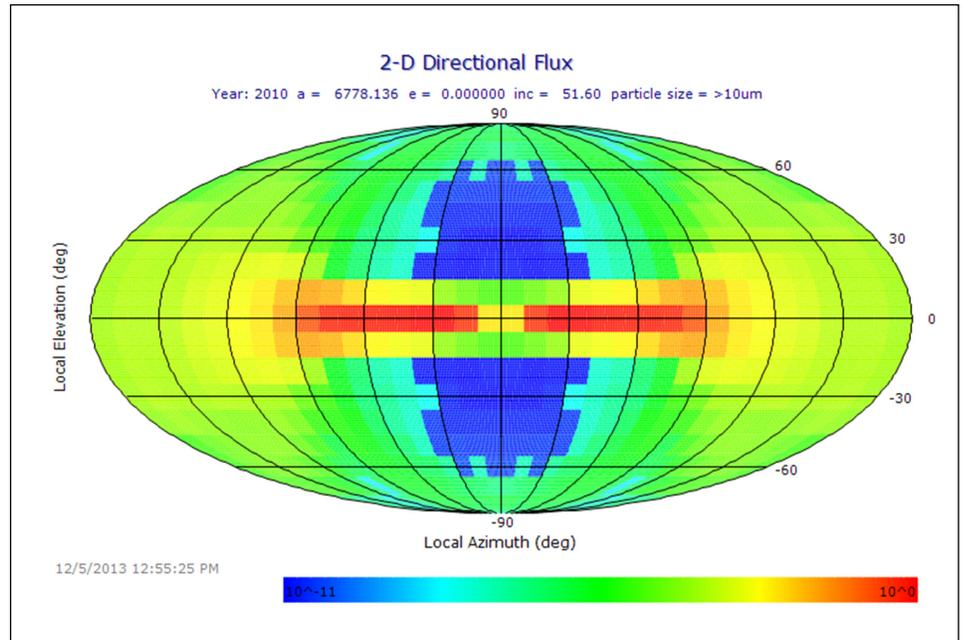
Figure 2. ORDEM 3.0 ISS 2-D flux chart (GUI output). Direction relative to the spacecraft is noted in (Local Azimuth, Local Elevation) coordinates: where Azimuth runs along the horizontal and ranges from [-180°, 180°], and Elevation runs vertically and ranges from [-90°, 90°]. Ram direction is defined by an (Azimuth, Elevation) of (0, 0), wake by (+180, 0), zenith by (Undefined, 90), and nadir by (Undefined, -90).
