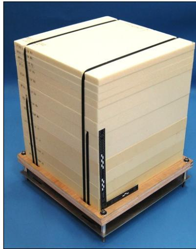
Figure 1. Soft-catch panel test article before impact.
