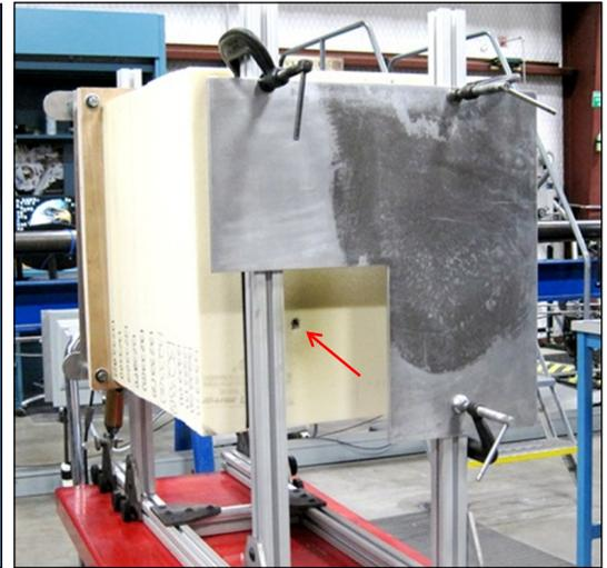
Figure 2. Test article outside the target chamber after the second impact. The entry hole damage is clearly visible to the lower left corner of the front panel, as indicated by the red arrow.
