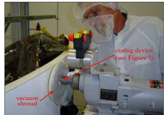
Figure 4. The vacuum shroud collects dust and chips during coring.
