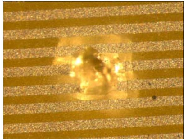
Figure 2. Damage caused by a 100  $\mu\text{m}$  glass particle, with an impact speed of 5 km/s, on a prototype RGS board.
