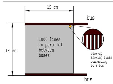
Figure 1. An illustration of the Resistive Grid Sensor.
