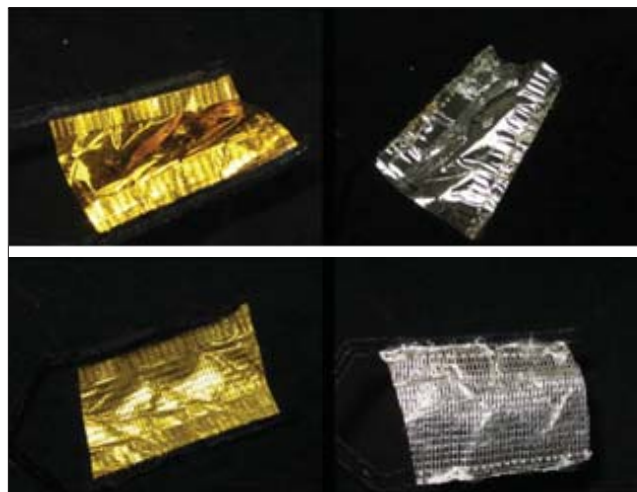
Figure 1. Digital Images of sample MLI debris. Top images are part of the space-facing layer and the bottom images are part of the space-craft facing layer. The A/m for these samples is ~ 10 m 2 /kg.
