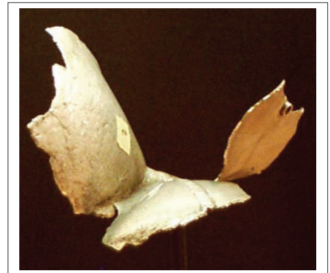
Figure 1. Image of Fragment 2 from the 6470 test. This is an example of a large crumpled fragment.
