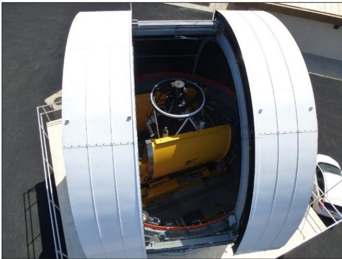
Figure 1. Interior view of the ES-MCAT showing the distinct hydrostatic bearing double-horseshoe equatorial mount.
