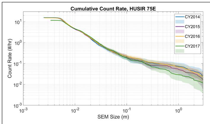
Fig. 4. Cumulative count rate for the orbital debris as a function of NASA SEM size. Shading color corresponds to CY line color.
