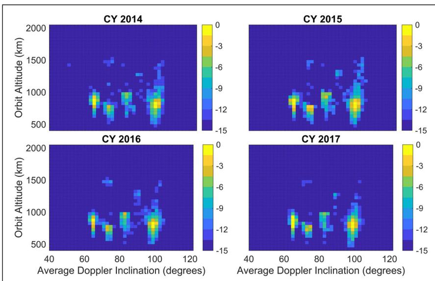
Fig. 3. Orbital debris count density in altitude (km) vs. Doppler-derived inclination ( $^{\circ}$ ) space. The color scale is in decibels (dB), hence each 3 dB decrease represents a factor of 2 decrease in count density.
