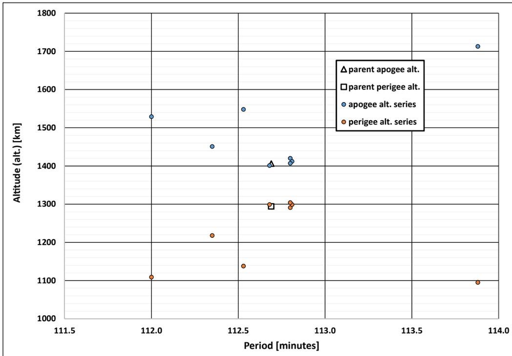
A Gabbard diagram of the 1992-052 third-stage event. Debris was injected into both longer and shorter-period orbits, indicating an energetic event.
