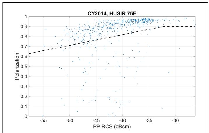
Fig. 6. Identification of the piecewise linear line that separates the NaK from the rest of the orbital debris population with altitudes < 1000 km and Doppler inclinations between  $62.9^\circ$  and  $67^\circ$ . The polarization shown is limited to positive values to highlight the NaK population, which has polarizations near unity.
