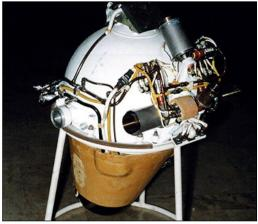
Figure 1. A SOZ unit with its 11D79 engine. Photo credit: RKK Energya/Kosmonavtika.com.
