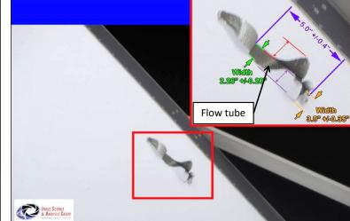
Figure 2. Close-up of exit damage.
