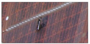
Figure 7. Another burned area in ISS Solar Array 3A (panel 42).
