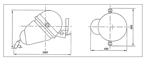
Figure 2. Plan views of a SOZ unit; all dimensions are in millimeters. Dry mass is 56 kg. Illustration from N. L. Johnson, "History of Soviet/Russian Satellite Fragmentations - A Joint US-Russian Investigation," Kaman Sciences Corporation, USA, October 1995, p. 19.
