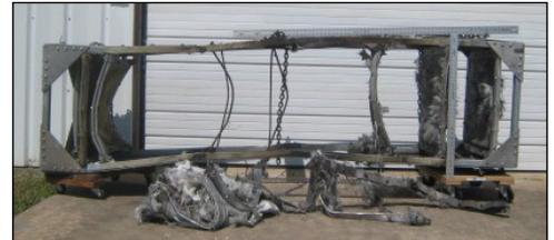
Figure 4. Post-test image of multi-shock shield target. First fiberglass bumper on right, Kevlar rear walls on left.
