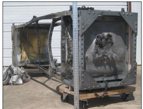
Figure 5. Post-test image of multi-shock shield. Front view of target.
