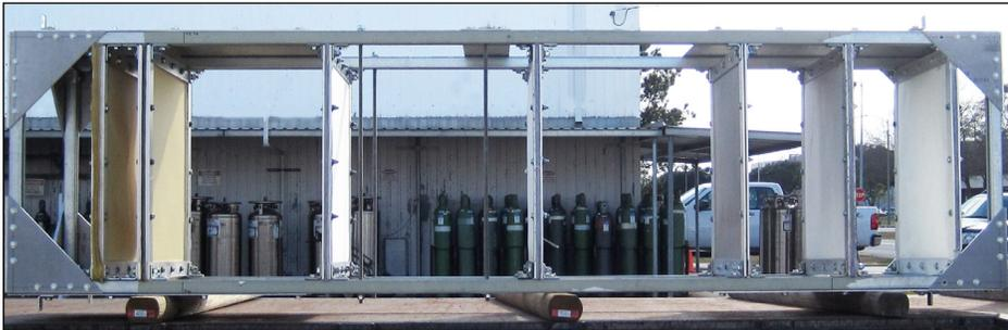
Figure 2. Pre-test image of multi-shock shield target. First fiberglass bumper is on right, Kevlar rear walls are on left.
