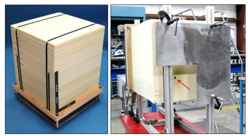
Figure 1. Soft-catch panel test article before Figure 2. Test article outside the target chamber after the second impact. The entry hole damage is clearly visible to the lower left corner of the front panel, as indicated by the
