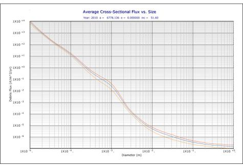
Figure 1. ORDEM 3.0 ISS debris diameter vs. cross sectional flux, with error bars (GUI output).
