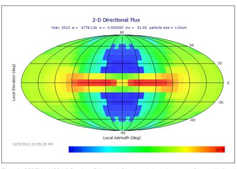
Figure 2. ORDEM 3.0 ISS 2-D flux chart (GUI output). Direction relative to the spacecraft is noted in (Local Azimuth, Local Elevation) coordinates: where Azimuth runs along the horizontal and ranges from [-180°, 180°], and Elevation runs vertically and ranges from [-90°, 90°]. Ram direction is defined by an (Azimuth, Elevation) of (0, 0), wake by (+180, 0), zenith by (Undefined, 90), and nadir by (Undefined, -90).
